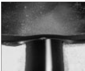
Even after 10,000 stress cycles on a section of membrane, this BITEC material showed no breakage or tearing.
