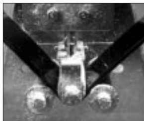
Bending tests performed at -22°F (-30°C) proved BITEC materials to be excellent for use in the coldest of climates.
