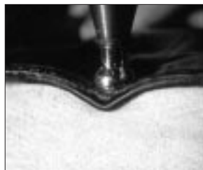
In repeated puncture tests, SBS membranes showed excellent resistance to penetration and perforation.
