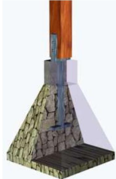
It is essential that a wood frame structure mounted on a concrete frame/brick stub wall must be fully anchored together. A bracket, as shown above left, made of non-corrodible metal, must be cast into the bearing structure to provide a structural connection for the whole wall through to the foundation. The wood column must be bolted to the bracket as shown, and the bracket must be fully secured into the concrete as shown on the right.
